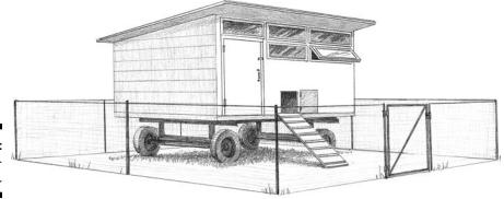
Figure 5-6: Mobile shelter with run.
