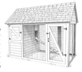
Figure 5-2: An all-inone chicken coop has a combined shelter and run.
